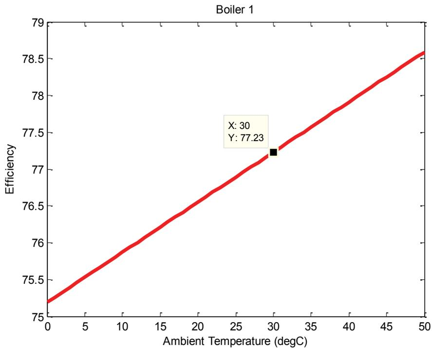
Fig. 4 Efficiency by different ambient temperature.
