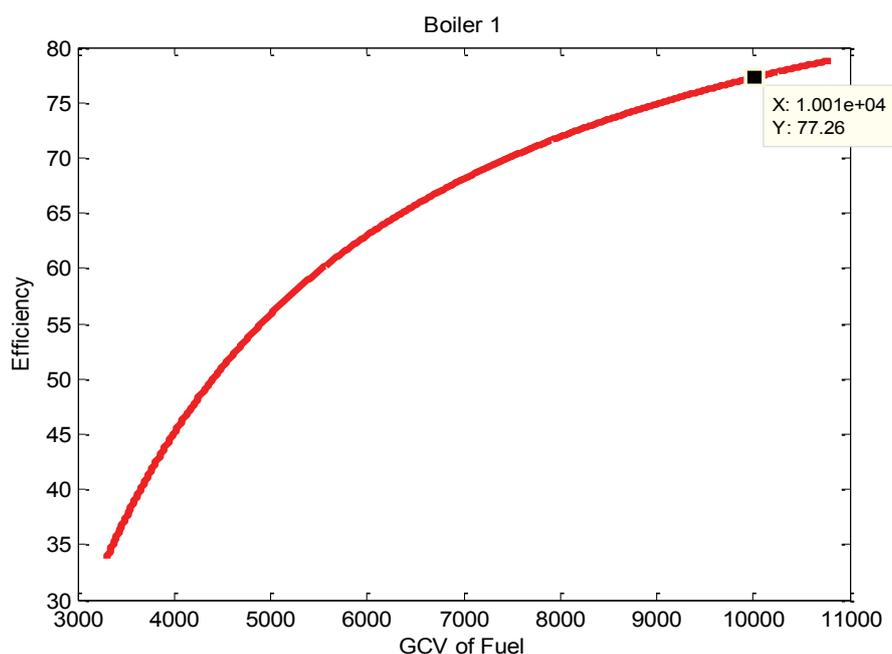
Fig. 2 Efficiency in different GCV of fuel.
