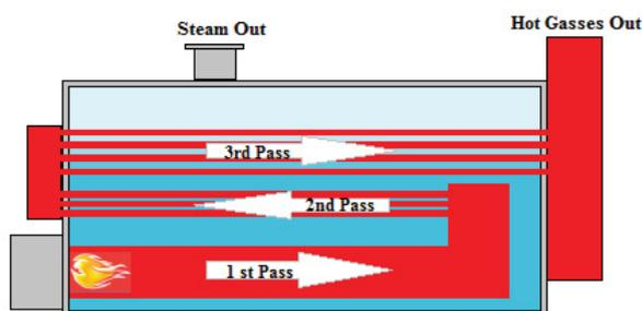
Fig. 1 Fire tube boiler gas flow (Ortiz, 2011).
