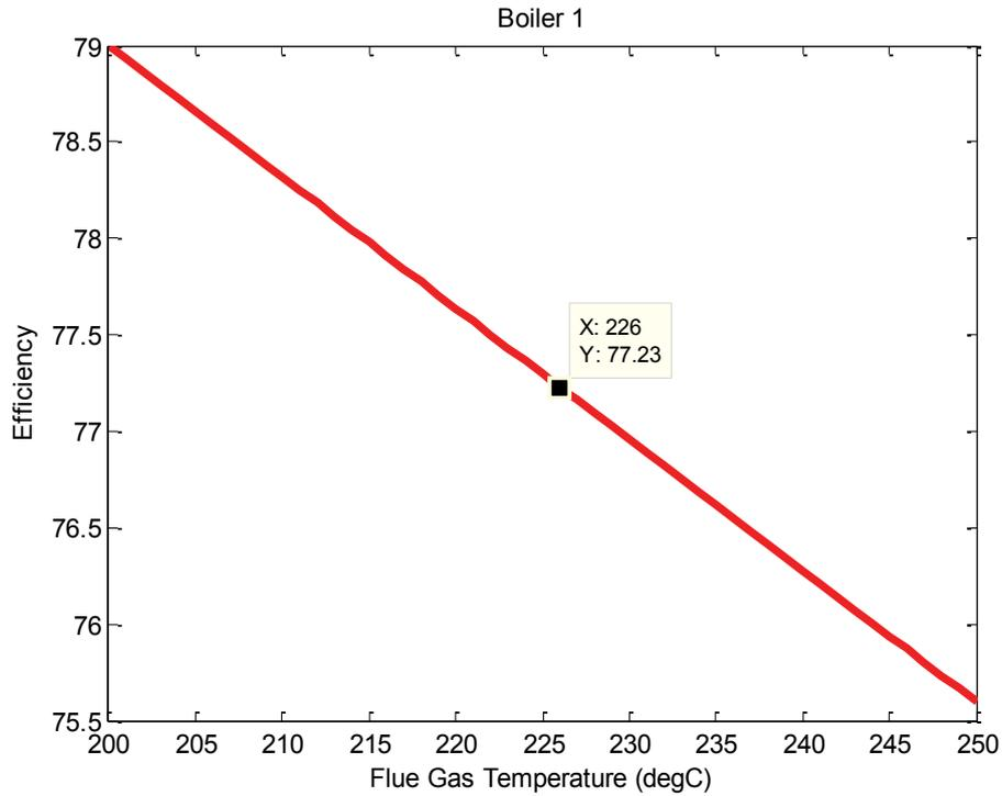
Fig. 3 Efficiency by different flue gas temperature.
