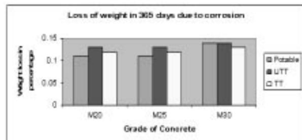
**Fig. 6** Loss of weight in 365 days due to corrosion after adding concare
