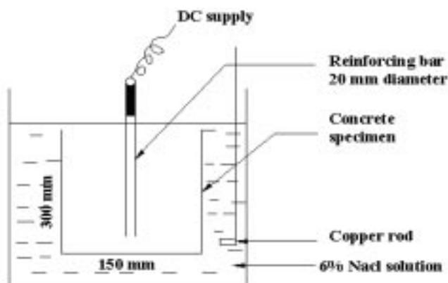
Fig.1 Accelerated corrosion test setup
