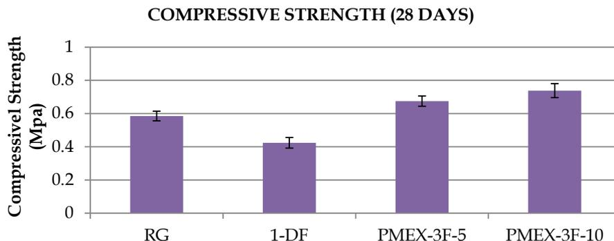
**Fig. 2** Compressive strength of lime mortar samples.
