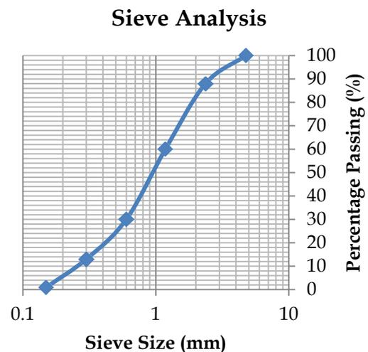
Fig. 1 Grain size distribution curve.
