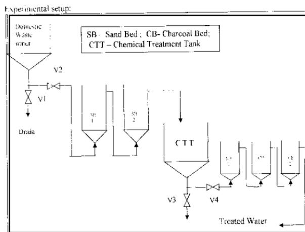
**Figure - 1 Domestic wastewater treatment unit**
