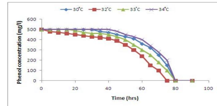
Fig. 1 Effect of Temperature on phenol degradation
