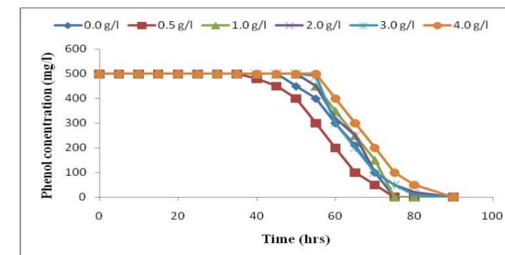
Fig. 2 Effect of glucose on phenol degradation
