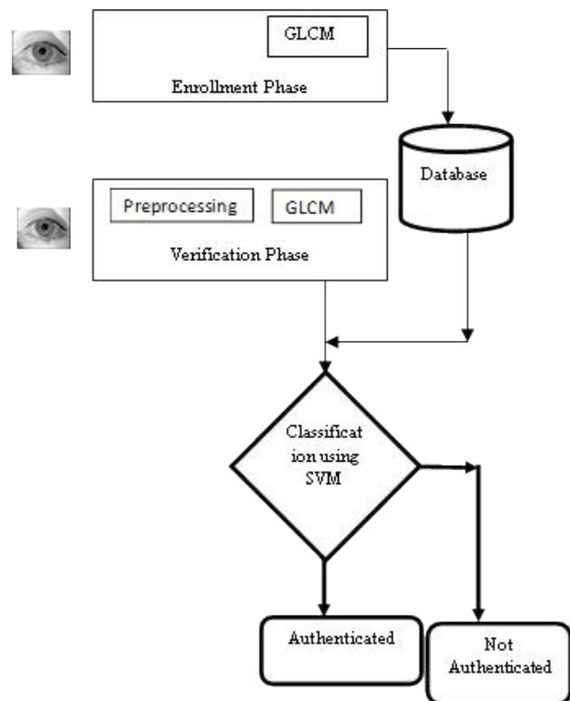
Fig.1 Block diagram of proposed iris recognition system.
