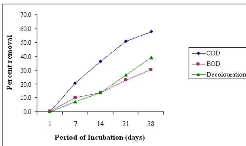
**Fig. 1** Percent removal of BOD and COD and colouration of textile effluents under aerobic condition
