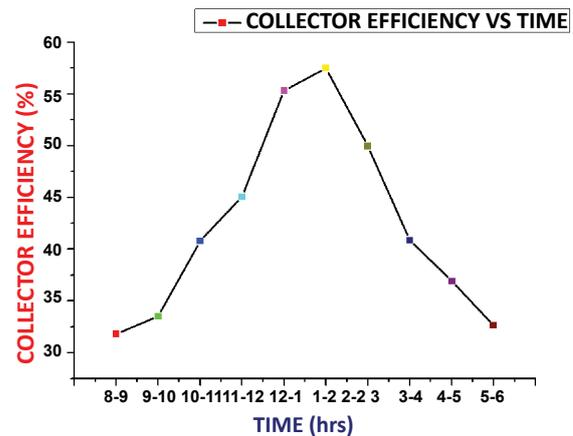
Fig. 2 The average values of collector efficiency vs. time for the evacuated solar air collector without absorber plate. The collector surface area=3.6  $\text{m}^2$ .
