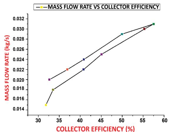
Fig. 4 The average values of mass flow rate vs. collector efficiency for the evacuated solar air collector without absorber plate. The collector surface area=3.6  $\text{m}^2$ .
