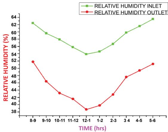
Fig. 5 The average values of relative humidity vs. time for the evacuated solar air collector without absorber plate. The collector surface area=3.6 m<sup>2</sup>.
