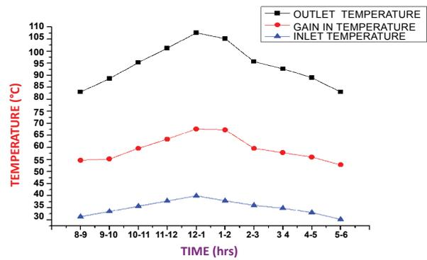
Fig. 8 The average values of temperature vs. time for the evacuated solar air collector with absorber plate. The collector surface area=3.6 m<sup>2</sup>.
