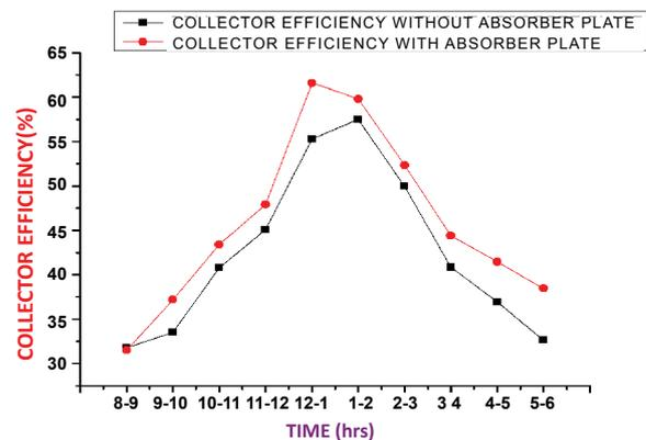
Fig. 10 The average values of collector efficiency vs. time for the evacuated solar air collector with and without absorber plate. The collector surface area=3.6 m<sup>2</sup>.
