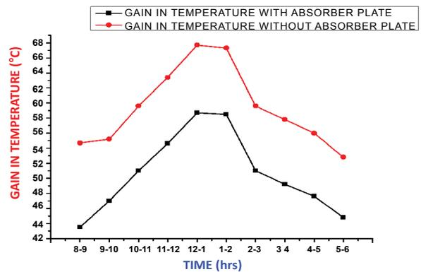
Fig. 9 The average values of gain in temperature vs. time for the evacuated solar air collector with and without absorber plate. The collector surface area=3.6 m<sup>2</sup>.
