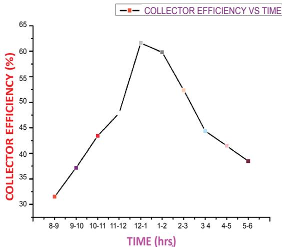
Fig. 7 The average values of collector efficiency vs. time for the evacuated solar air collector with absorber plate. The collector surface area=3.6 m<sup>2</sup>.
