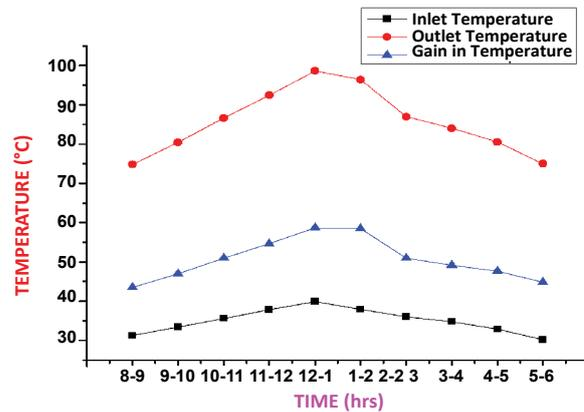
Fig. 3 The average values of temperature vs. time for the evacuated solar air collector without absorber plate. The collector surface area=3.6  $\text{m}^2$ .
