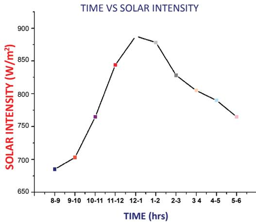
Fig. 6 The average values of solar intensity vs. time for the evacuated solar air collector without absorber plate. The collector surface area=3.6 m<sup>2</sup>.
