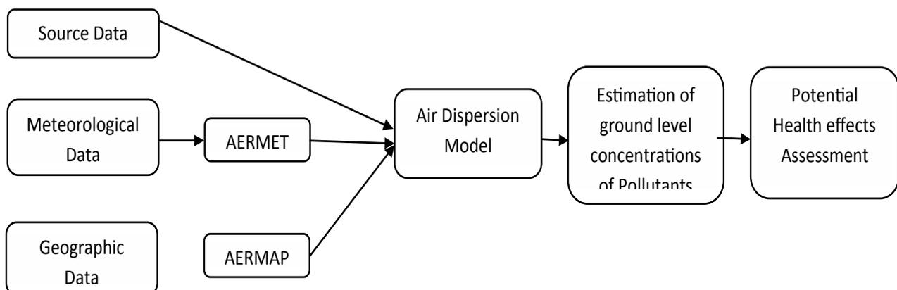
**Fig. 1** AERMOD Dispersion Modeling Flow Diagram.
