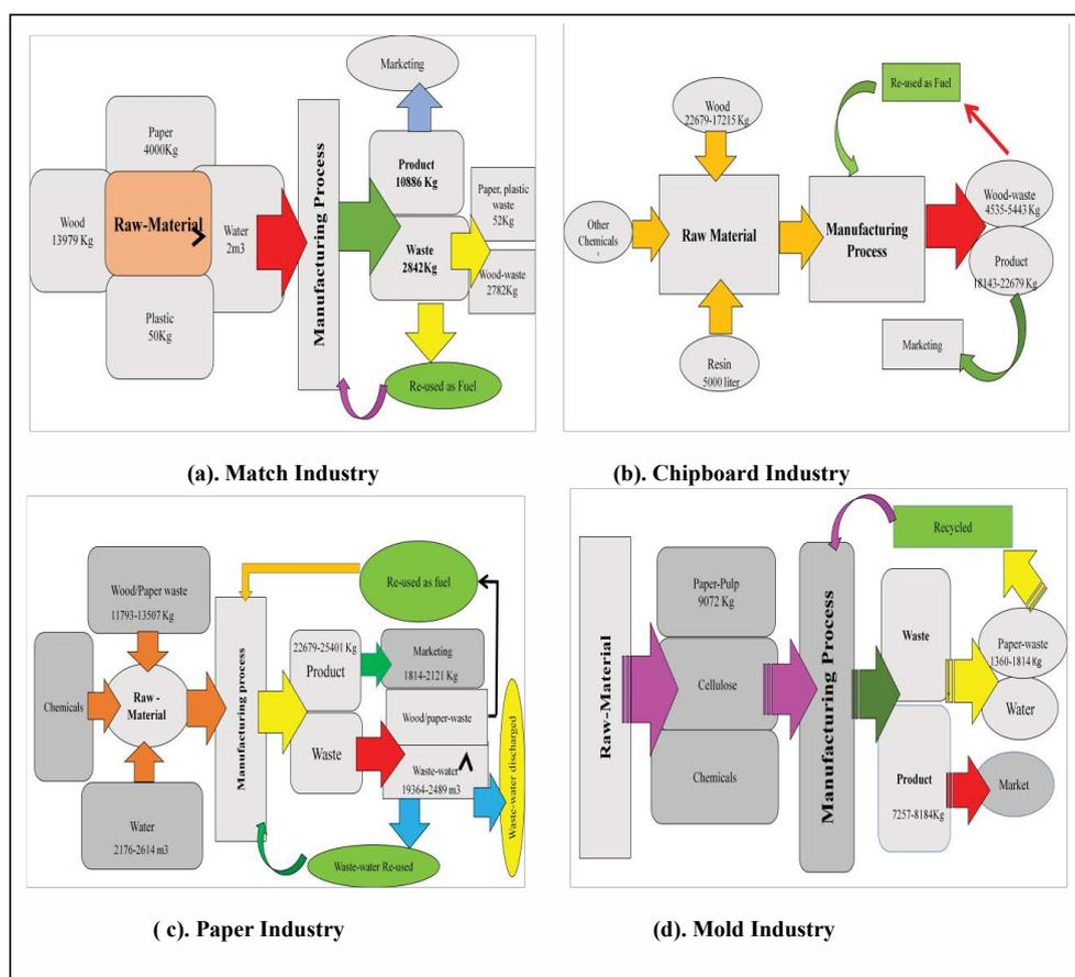
Fig. 2 Manufacturing process of selected industries.
