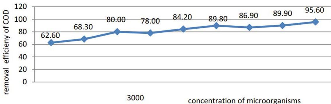
Fig 9. The diagram for the removal efficiency of COD versus concentration of microorganisms.
