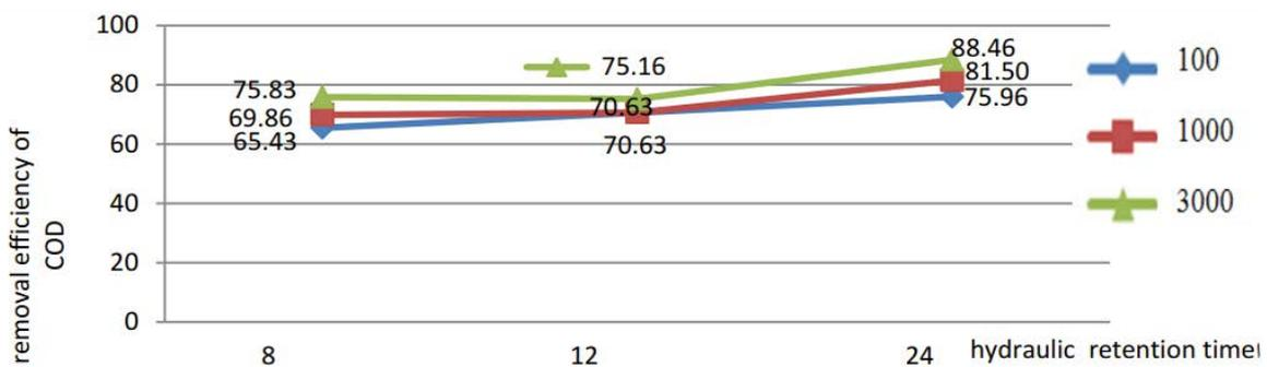
Fig 7. The diagram for the removal efficiency of COD versus hydraulic retention time by individual concentration of microorganisms.
