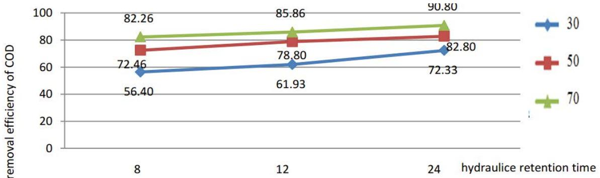
Fig 8. The removal efficiency of COD versus hydraulic retention time by individual filling percentage.
