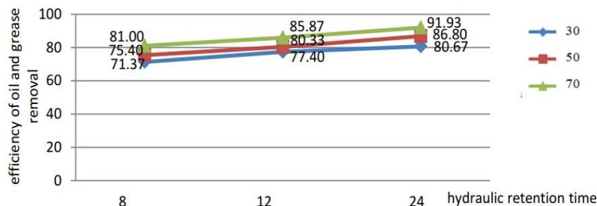
**Fig 4.** The diagram of efficiency of oil and grease removal versus hydraulic retention time by individual concentration of microorganisms.
