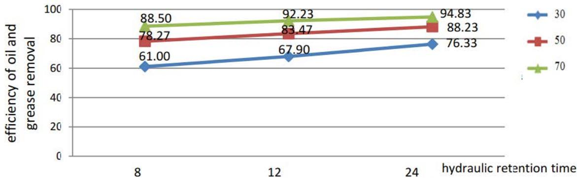
Fig 5. The diagram of efficiency of oil and grease removal versus hydraulic retention time by individual filling percentage.
