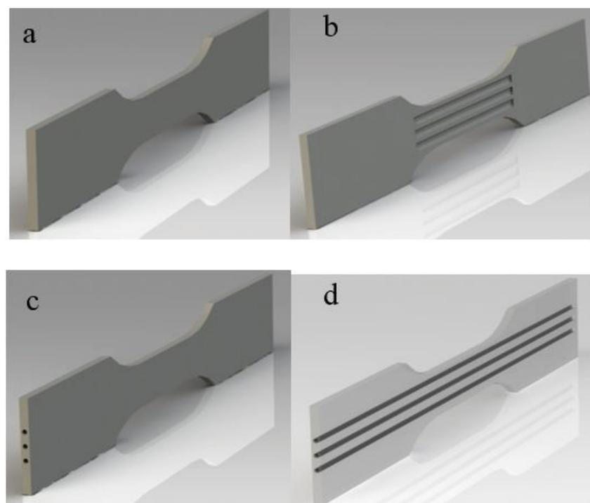
**Fig. 1** Three-dimensional models of synthesized samples (a is a standard sample, b is a sample with a relief on the surface, c is a sample with internal channels, and d is a longitudinal section of the sample with channels).
