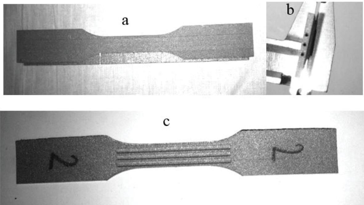
**Fig. 2** Type of synthesized samples (a – sample with internal channels before removal of technological support, b – cross section of synthesized sample with channels, c – sample with relief on surface after removal of technological support).
