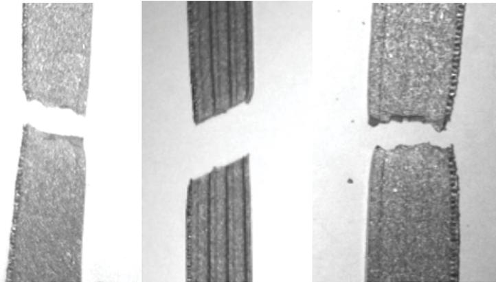
**Fig. 5** The nature of the destruction of the samples (a is a sample of a solid material, b is a sample with a relief, and c is a sample with internal channels).
