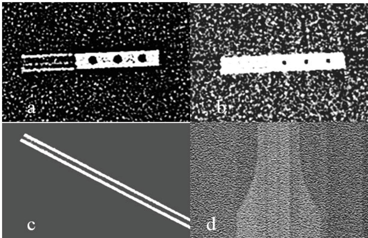
Fig. 3 Results of the investigation of the internal structure of the samples with channels on the VT-600X A tomograph (a is the low-frequency reconstruction of the cross section, b is the high-frequency reconstruction of the cross section, c is the tomography of the longitudinal section of the sample, and r is the x-ray diffraction pattern of the sample in the plane).
