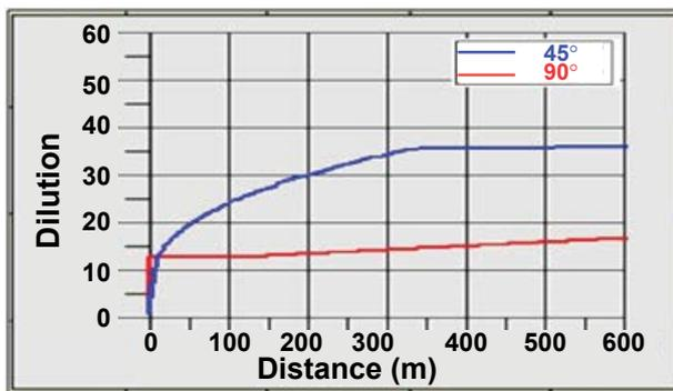
**Fig. 7** Graph of dilutions according to different diffuser inclinations.
