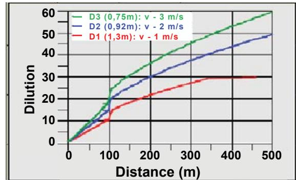
**Fig. 9** Dilutions graphs according to different diffuser diameters.
