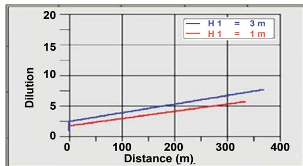
**Fig. 6** Graph of dilutions according to different stack heights.
