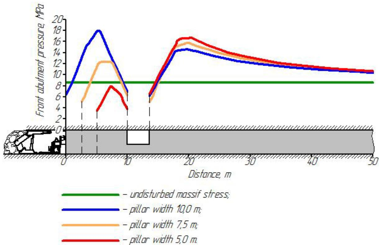
Fig. 5 Distribution of bearing pressure ahead of the mining face at the different stages of the mining face approaching the advanced mine working.
