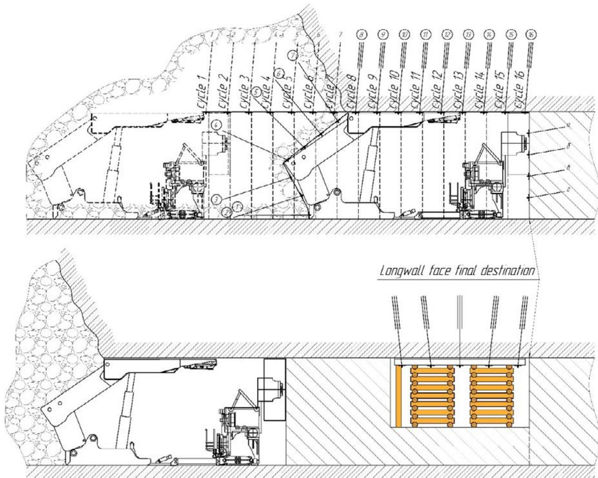
Fig. 1 Diagram of dismantle chamber forming via inserting the longwall set of equipment into a previously sunk mine working.
