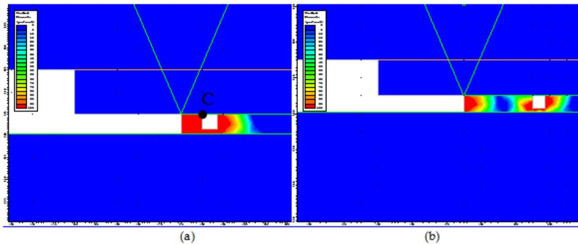
Fig. 4 Field of deformation distribution in the vicinity of the dismantling area for the pillar between the longwall and preliminary sunk mine working having the width of 5 m (a), 10 m (b).
