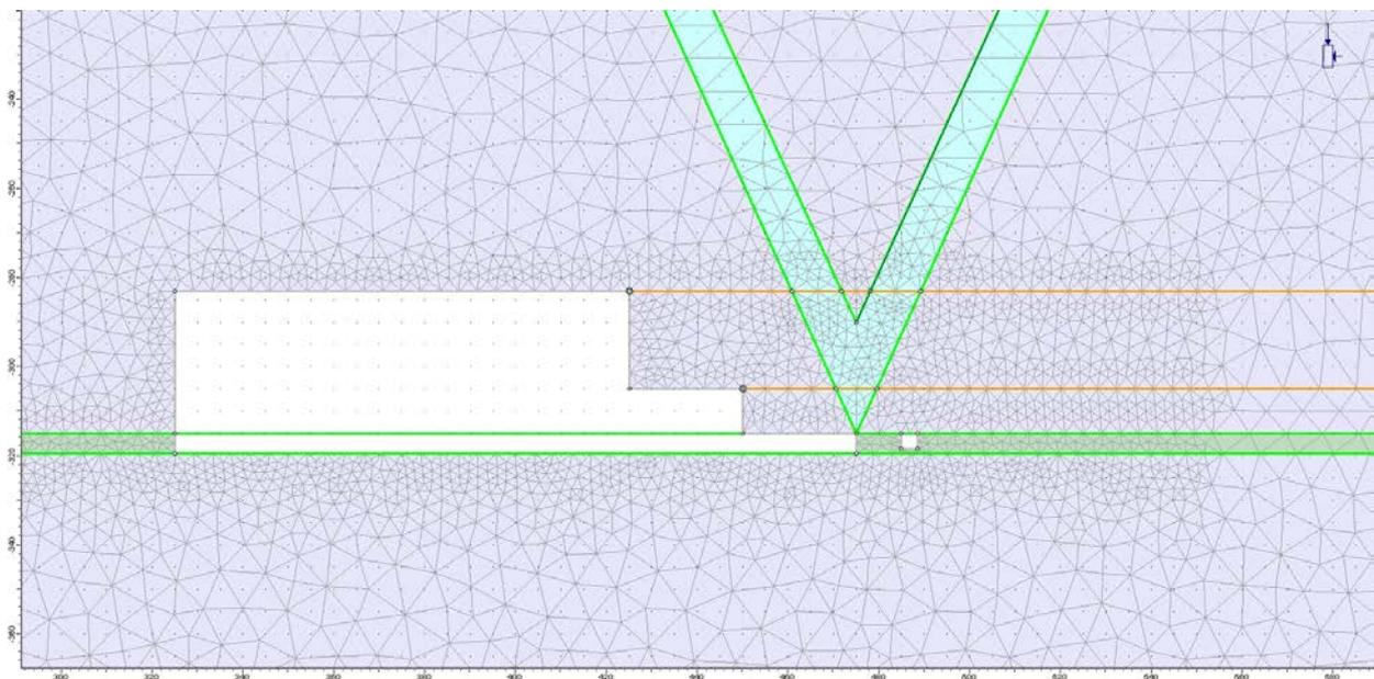
Fig. 2 Mining and mechanical model of rock massif in mining face approaching the dismantling area.
