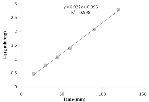
Fig. 6 Second order kinetic of adsorption of COD<sub>residual</sub> from flax wastewater.
