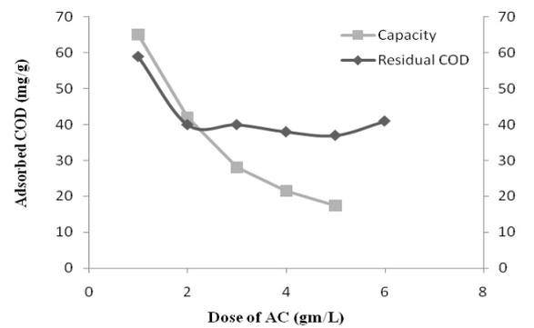
Fig. 4 Effect of adsorbent dosage on COD removal.
