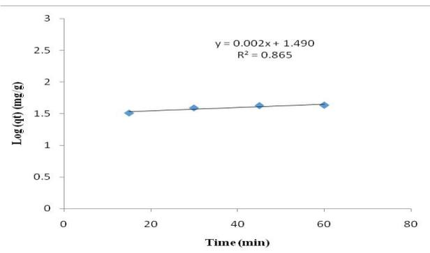
Fig. 5 First order kinetic of adsorption of COD<sub>residual</sub> from Flax wastewater.
