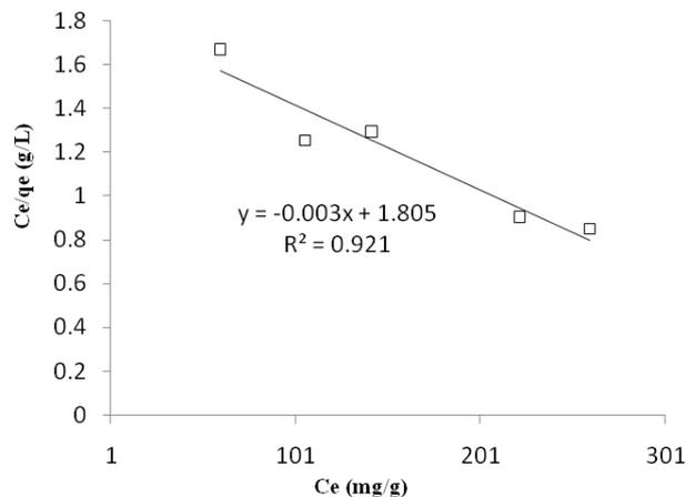
Fig. 7 Langmuir isotherm model of COD removal over AC.
