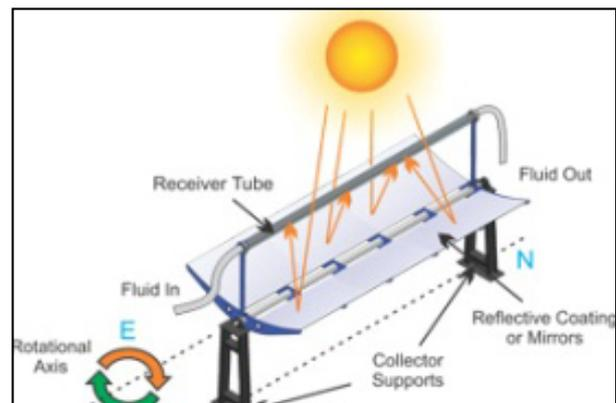
Fig. 1 Parabolic through collector.
