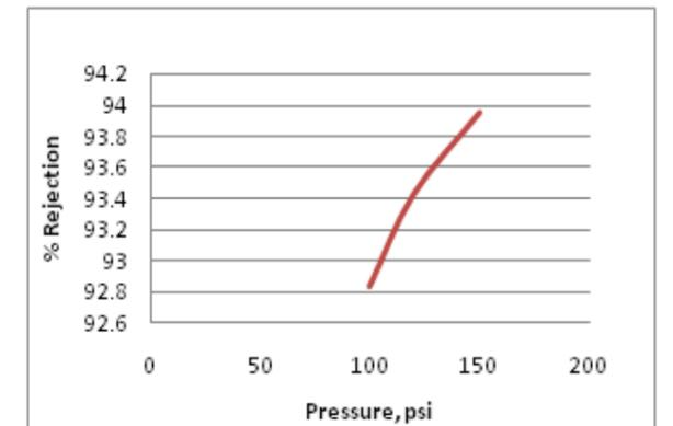
Fig. 11 Effects on % rejection on different applying pressure
