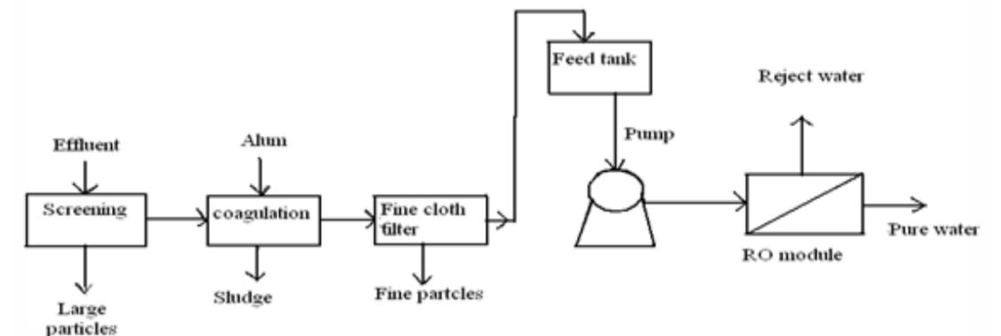
Fig. 1 Process flow diagram of treatment of tannery wastewater
