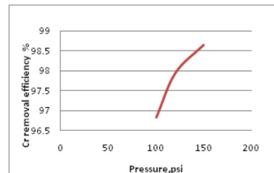
Fig. 9 Effects of chromium removal efficiency on different applying pressure
