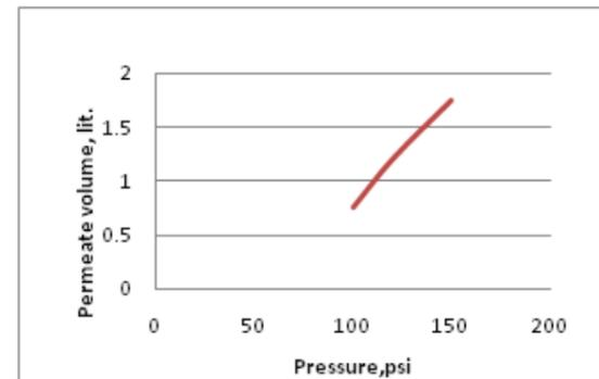
Fig. 7 Effects of permeate volume on different applying pressure
