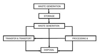
**Fig. 2.** Flow chart shows the inter relationship between functional elements in solid waste management.
