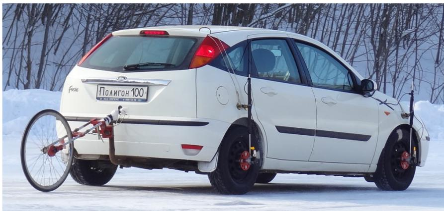
Fig. 3 Test vehicle ford focus I.
