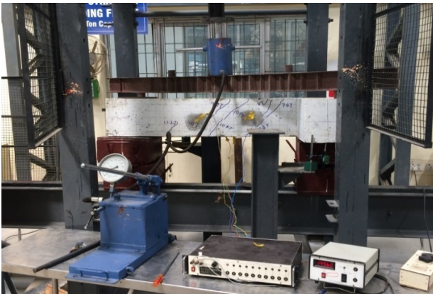
Fig. 5 Torsion test on conventional beam.
