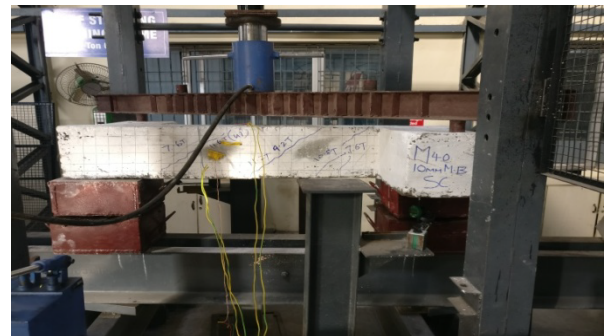
Fig. 7 Torsion test on special concrete beams.
