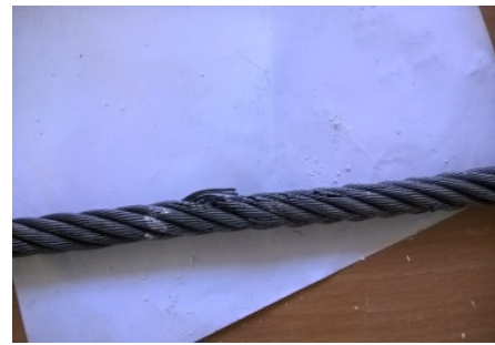
Fig. 2 Steel cable after failure.
