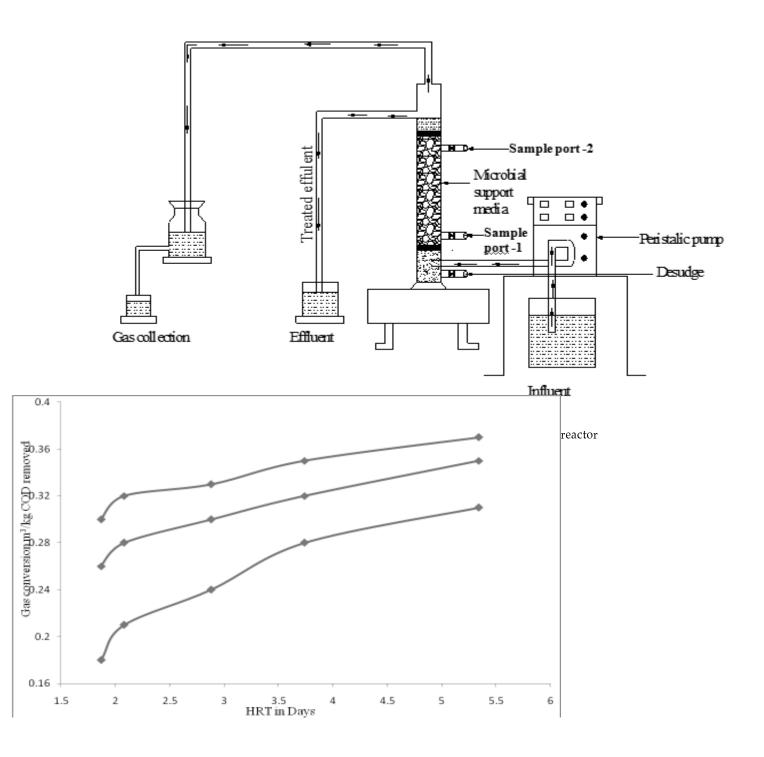
Fig. 2 HRT in Days Vs Gas conversion m3/kg COD removed for an average COD of 2072mg/1,2608mg/1,3024mg/L.
