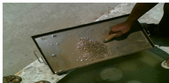
Fig. 3 Soaking of the recycled coarse aggregates in cement fly ash mixture.
