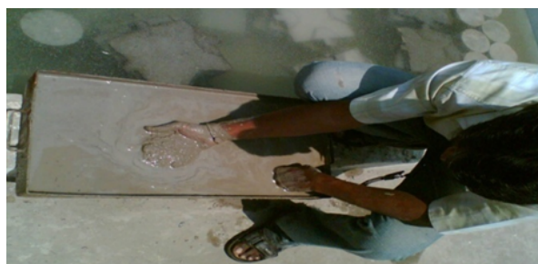
Fig. 4 Soaking of the recycled fine aggregates in cement fly ash mixture.
