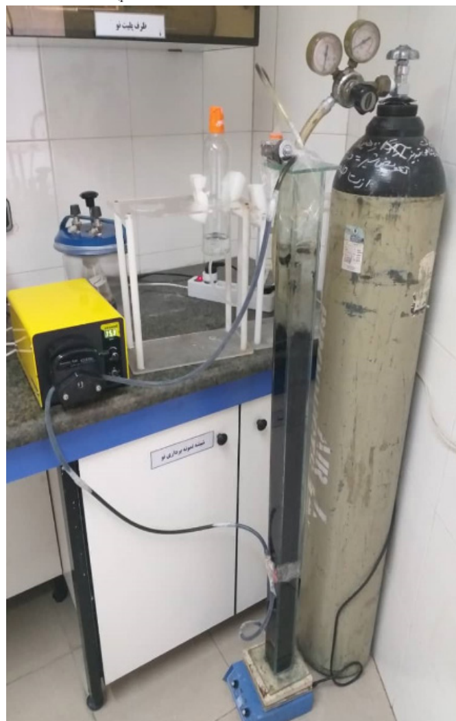
Fig. 3 The setup of a down-flow fluidized bed bioreactor on a laboratory scale.
