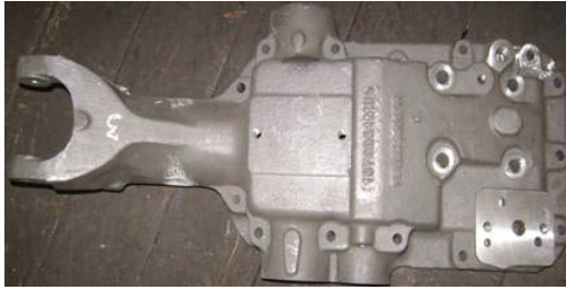
Fig. 6 Hydraulic lift cover.
