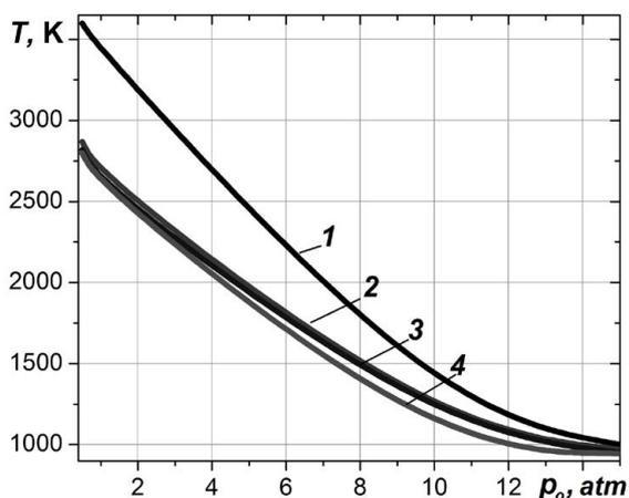
Fig. 4 Dependence of temperature of plasma channel from the pressure inside the plasma chemical reactor at different distances from the electrode: 1 cm to 2 cm, 2 cm to 9 cm, 3 cm to 17 cm and 4 cm to 25 cm.
