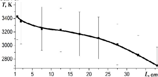
Fig. 1 The distributions of the dispersed phase of the temperature along the axis of the plasma channel.
