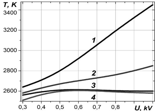
Fig. 2 Dependence of temperature of plasma channel from magnitude of the supply voltage at different distances from the electrode: 1 cm to 2 cm, 2 cm to 9 cm, 3 cm to 17 cm and 4 cm to 25 cm.
