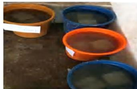
Fig. 1 Specimens Immersed in ( H_2SO_4 ) Solution
