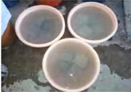
Fig. 2 Specimens Immersed in (Na 2 SO 4 ) Solution
