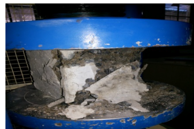
Fig. 2 Compressive strength testing.
