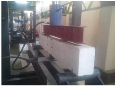
Fig. 3 Beam for flexural strength testing.
