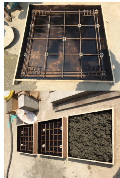
Fig. 2 (a) Casting of slab panels. (b) Variations in compressive strength of concrete.
