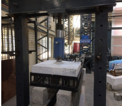
Fig. 3 Testing of slab panel.
