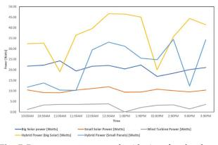
**Fig. 7** Power output measured with time for the three individual renewable energy systems compared with the two hybrid systems.
