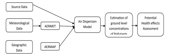
Fig. 1 AERMOD Dispersion Modeling Flow Diagram.
