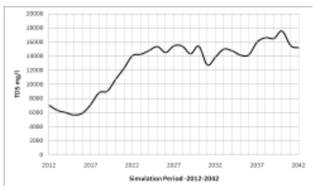
Fig. 18 Variation of TDS in 30 years of simulation period in Ambur village without any remediation
