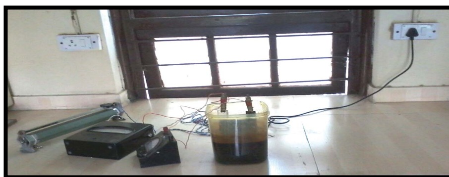
Fig. 1 Lab scale electro-coagulation set-up.
