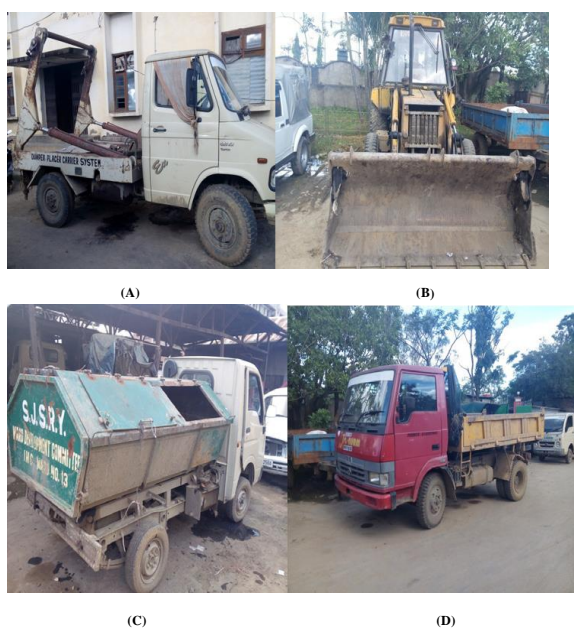
Fig. 2 (A), (C) and (D) Vehicles are used for collection, transportation and disposal of waste; (B) Vehicle used for loading/unloading of waste in landfill.
