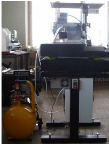
Fig. 5 Mock-up machine with complete vibration insulation.
