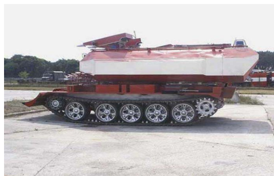
Fig. 2 Czech caterpillar fire machine SPOT-55 equipped with a pair of water guns. The water expense is 2 \times 40 l/s or 2 \times 70 l/s, the distance is up to 50 m, a TV-camera is used for remote control of the water-guns, the water tank capacity is 12 tons of water and 1 ton of foam.
