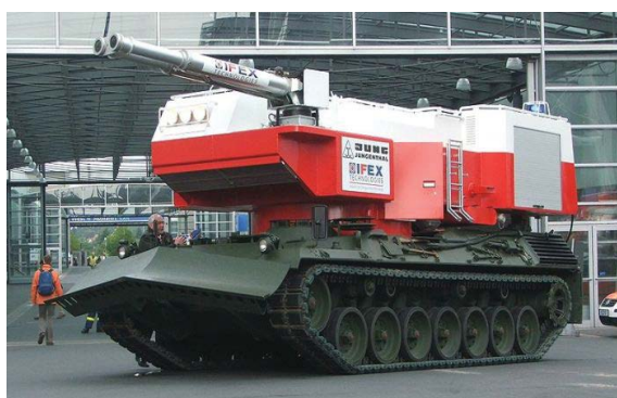
Fig. 6 German IFEX module with paired barrels based on a “Leopard-1” tank chassis. Pneumatic impulse volley of 40 liters of water spray to the distance up to 40 m, capacity – 10 tons of water, high pressure compressor.
