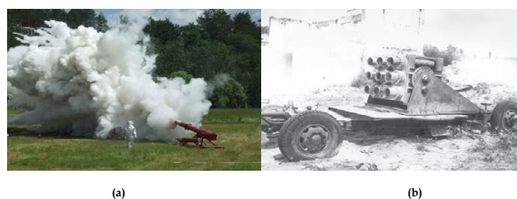
Fig. 3 a) single-barrel pneumatic impulse module mounted at sledges, industrially produced since 1987 for emergency gas-wells brigades; the system pulverizes 200 kg of extinguishing powder to 25 m and has an extinguishing range up to 15 m, total extinguishing area – up to 60 m 2 along trajectory. b) Module MM-9 mounted at gun-carriage; its volley pulverizes 180 kgs of the same powder up to 90 m with fire extinguishing range up to 60 m and a total extinguishing area of up to 550 m 2 along the trajectory. These 20 MM-9 modules have operated at Chernobyl area since June 1986 as fixed elements of an automatic remote-control fire system. Each module protected area equal to 300 m 2 to 800 m 2 .
