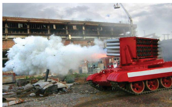
Fig. 5 Firefighting system MM-50 during hotbed extinguishing in an industrial area by artificial vortex through open gates, doors and windows.
