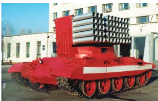
Fig. 1 Caterpillar fire machine "Impulse-3M" with a 50-barrel tower module; 20 kg - 25 kg of extinguishing agent is in the channel of each barrel; firefighting characteristics: distance - up to 110 m, area - up to 1000 m 2 /s for the volley from 10 barrels, total area covered by 5 volleys - up to 3000 m 2 to 5000 m 2 . The machine was designed and produced during the last years of the USSR by V.D. Zakhmatov's scientific group.
