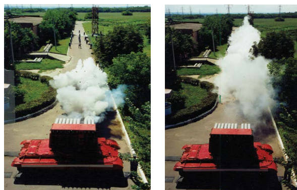
Fig. 4 a) Firefighting system MM-50: a 10-barrel volley spreads an extinguishing gas-powder hurricane to a distance of 60 m to 110 m to stop a "terrorist" (played by volunteers) attack, time is 0.18 s. after the initiation of the volley; b) the hurricane coverage area of 12 m long and 4 m to 12 m wide, the total area is over 1000 m 2 , and the time is 1.8 s. after the initiation of the volley.
