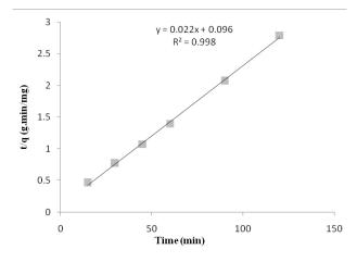
Fig. 6 Second order kinetic of adsorption of  $\text{COD}_{\text{residual}}$  from flax wastewater.
