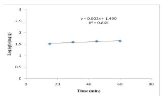
Fig. 5 First order kinetic of adsorption of  $COD_{residual}$  from Flax wastewater.
