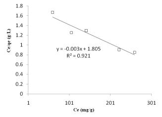
Fig. 7 Langmuir isotherm model of COD removal over AC.
