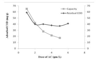
Fig. 4 Effect of adsorbent dosage on COD removal.
