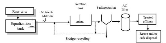
Fig. 1 Flow diagram of the treatment process.
