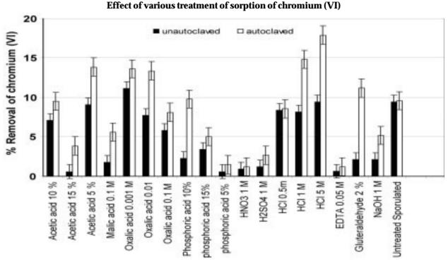
Fig. 1 Effect of autoclaving on chemically treated dead sporulated biomass of *A.niger* in the sorption of Chromium (VI) ions
