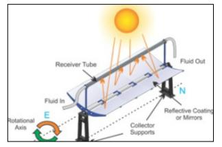
Fig. 1 Parabolic through collector.
