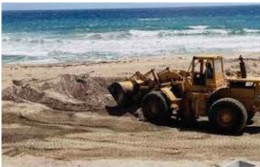
Fig. 2 Mechanized mining of garnet sand.
