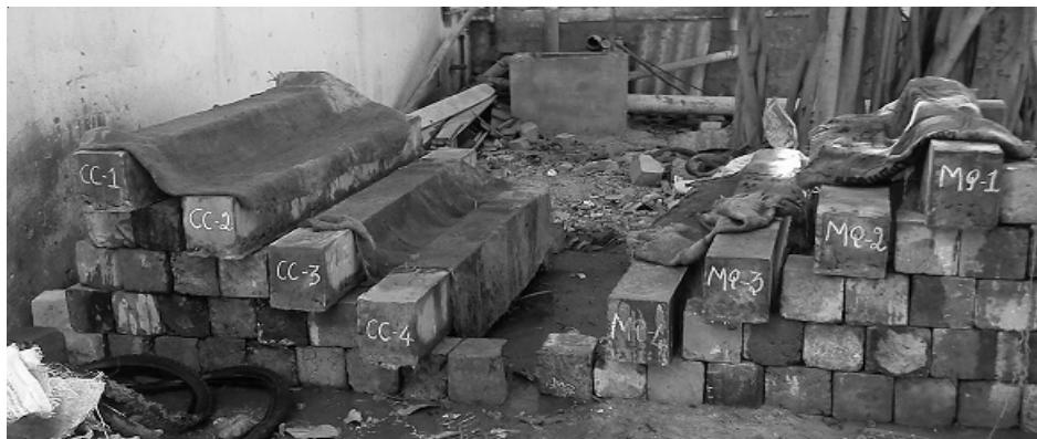
**Fig. 5** Test specimens Flexure beam under Curing
