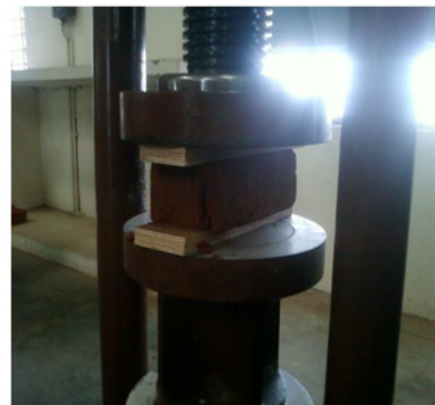
Fig. 1 Compressive strength of conventional bricks
