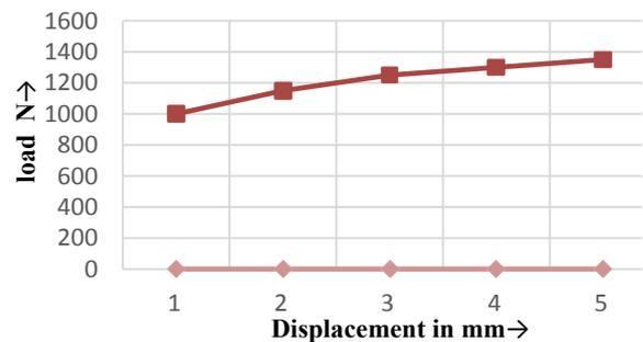
Fig. 14 Load v/s displacement curve (K-joint).
