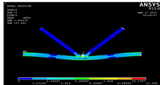
Fig. 12 Stress distribution of K-joint.
