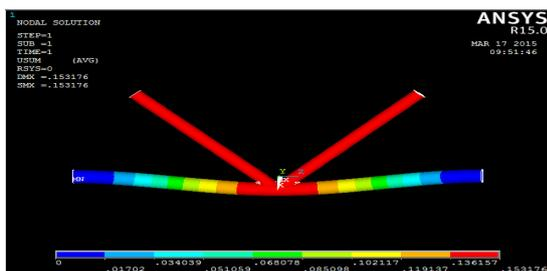
Fig. 10 Displacement of K-joint.
