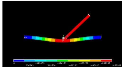
Fig. 11 Displacement of Y-joint.
