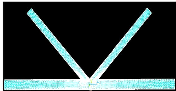
Fig. 6 Meshing of K-joint.
