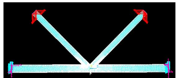
Fig. 8 Loading of Y-joint.
