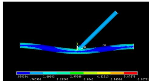
Fig. 13 Stress distribution of Y-joint.
