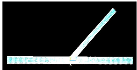
Fig. 7 Meshing of Y-joint.
