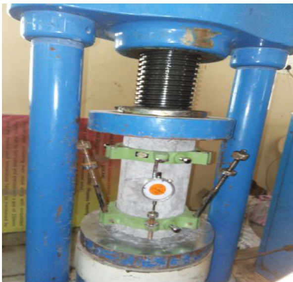
Fig. 2 Column specimen fix for testing.
