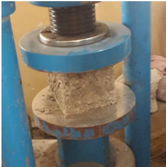
Fig. 1 Cube sample in CTM.
