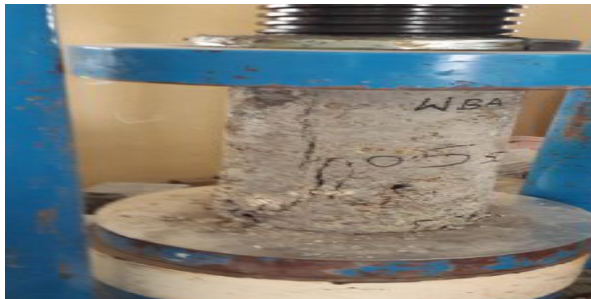
Fig. 3 Cylinder specimen after failure.
