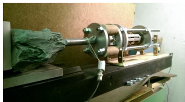
Fig. 3 Installation for studying the propagation of shock waves in the clay.
